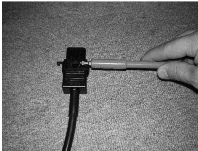
Figure 1.5. Loosen the Clamp on the Cable.
