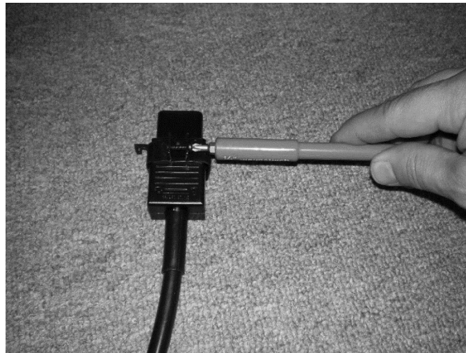
Figure 1.11. Loosen the Clamp on the Cable.
