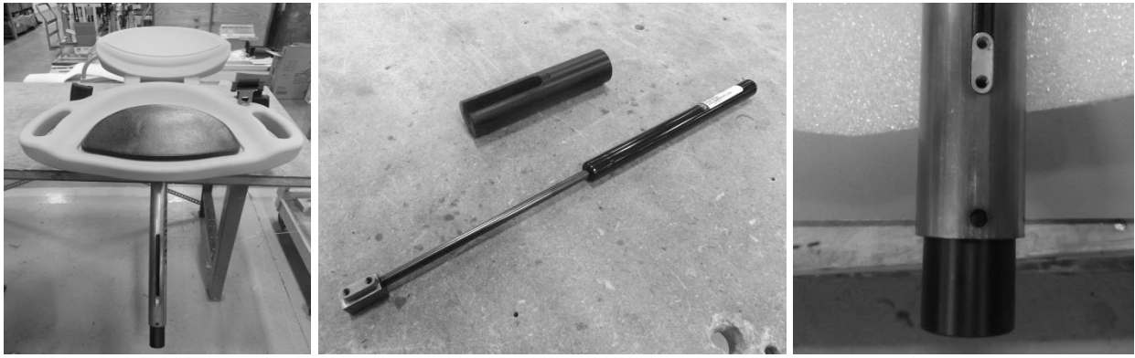
Figure 2.3. Gas Spring/Mounting Block Stopper (Left), Gas Spring with Mounting Block (Center), and Mounting Block Stopper (Right).
