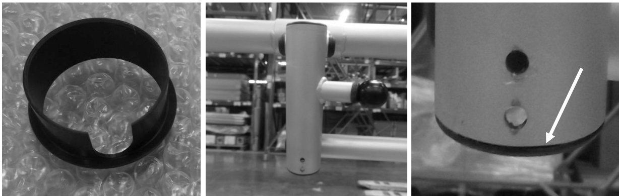
Figure 2.4. Bushing Front Guide with Cutout (Left), Seat Female Tube Assembly (Center), Bushing Glued into Bottom of Tube (Right).
