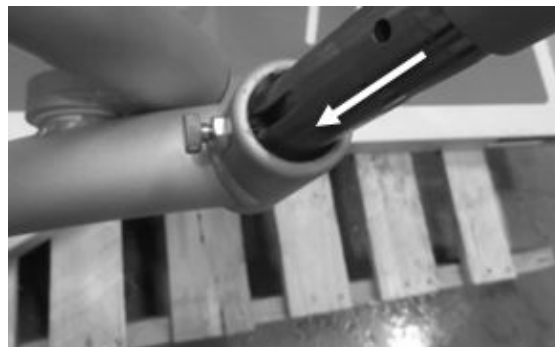
Figure 2.2. Align Plunger with Handle Groove, Insert Handle Assembly, and Tighten Screw.
