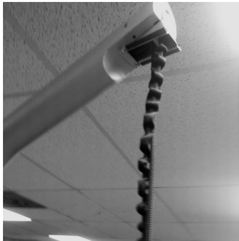
The Figure 3.11. The safety tether (the rippled elastic cord) attaches to the center of the patient harness bar.
