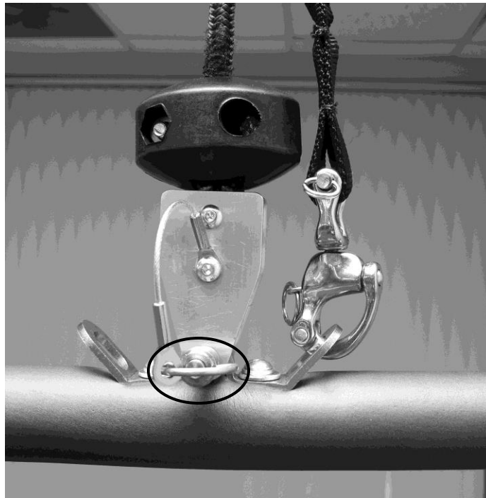
Figure 3.2. Quick Disconnect Apparatus Illustrating Quick Release Pin.
