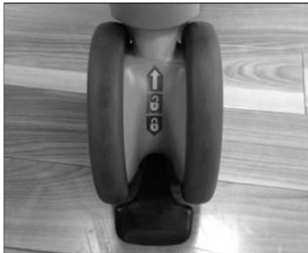
Figure 3.4. The front casters have three setting: completely locked, completely unlocked, and directionally locked.
